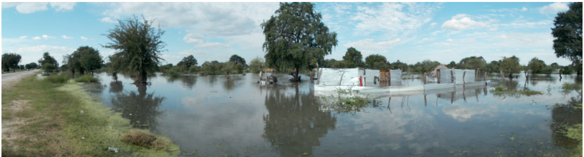
Figure 26: An example of flooded buildings which were constructed in seasonal watercourses (a) and near seasonal water courses with dyke roads blocking the water flow in the Cuvelai Basin (b)
